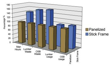
Figure 1. Relative comparison between panelized and stick framing technologies
